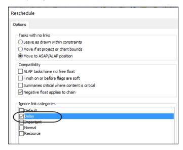
• Then the Delay tasks are ignored in the schedule calculation resulting in a Collapsed schedule:
